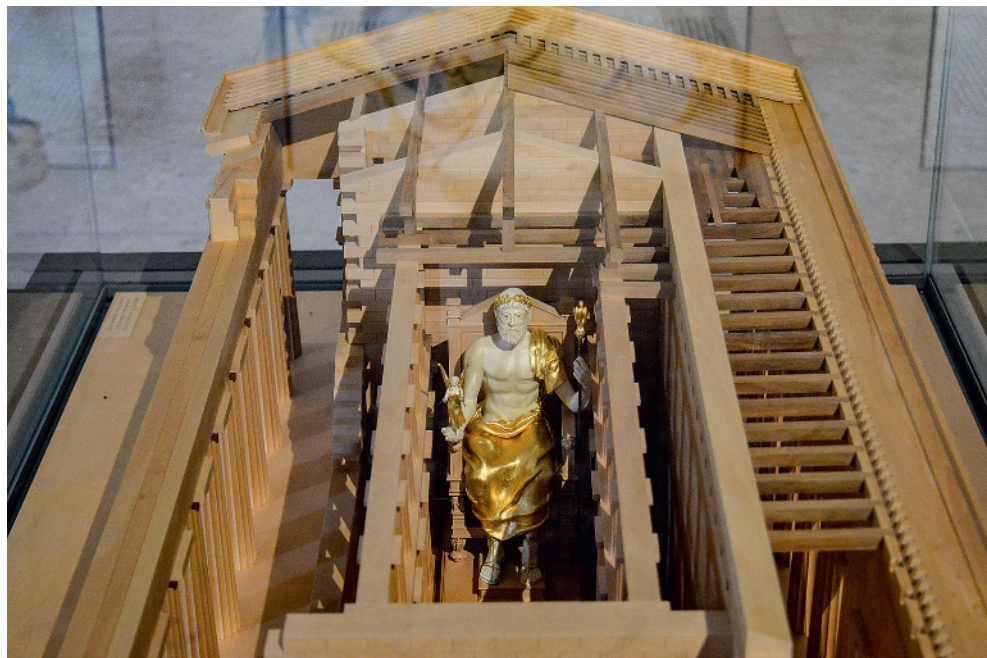
Figure 1.4 Cutaway model of the temple of Zeus that shows some of the wooden rafter structure.
