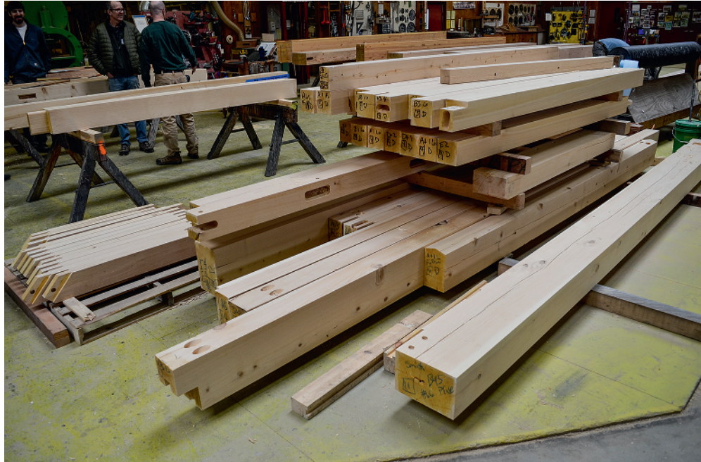
Figure 1.20 Various contemporary glulam beams in a shop.
