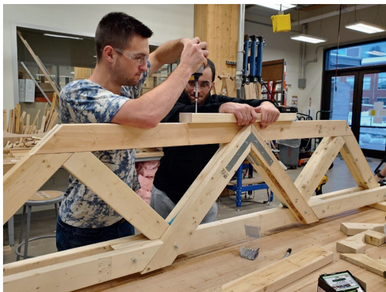
Figure 1.28 Hands-on projects that allow students to design, fabricate, and test wooden structural components are helpful to reinforce understanding of the material.
