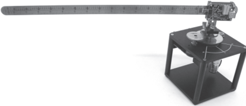
Figure 1.4 A single-link flexible manipulator system.
