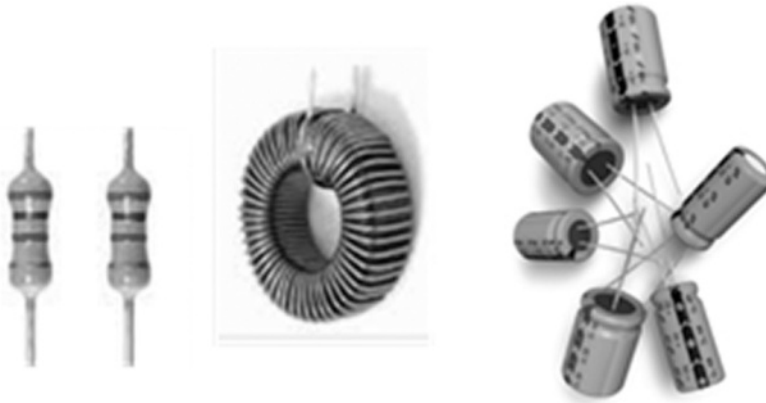
Figure 1.28 Simple passive electronic components are used to filter out the interference.
