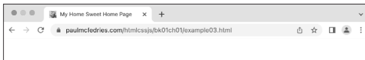
FIGURE 1-2: The text you insert into the <title> tag shows up in the browser tab.
