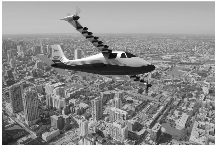
■ FIGURE 1.46 NASA X-57 all- electric distributed propulsion flight demonstrator. (Source: Courtesy of NASA)
