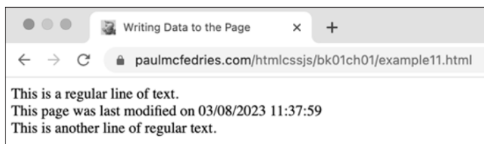
FIGURE 1-2: When you open the file, the text displays the date and time the file was last modified.
