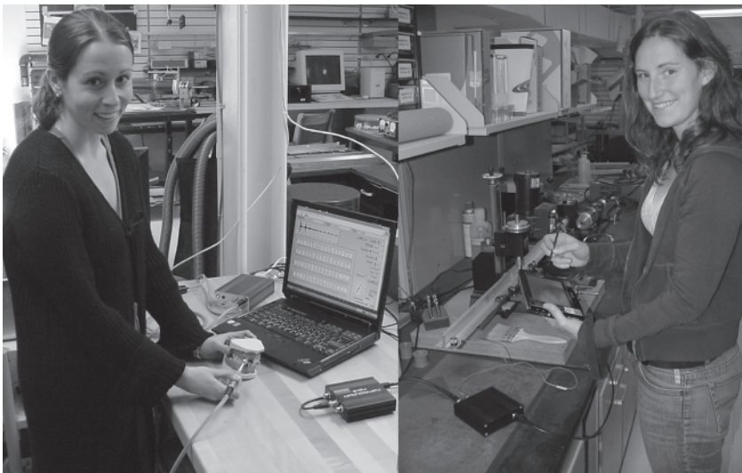
Figure 1.8 In recent years, both the computers and the ultrasonic instrumentation have shrunk dramatically. A tablet or laptop controls a USB-powered nanopulser , which is a combined pulser-receiver and A/D unit connected to a contact transducer or handpiece.
