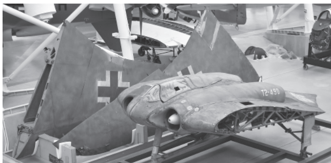
Figure 1.18 The Horten [65] flying wing would have been quite stealthy even if its wings weren't made from plywood. After the war, Reimar Horten said he mixed charcoal dust with wood glue to absorb radar and shield the aircraft from detection by British radar that operated at 20–30 MHz. Source: HawkeyeUK/Wikimedia Commons/CC BY-SA 2.0.
