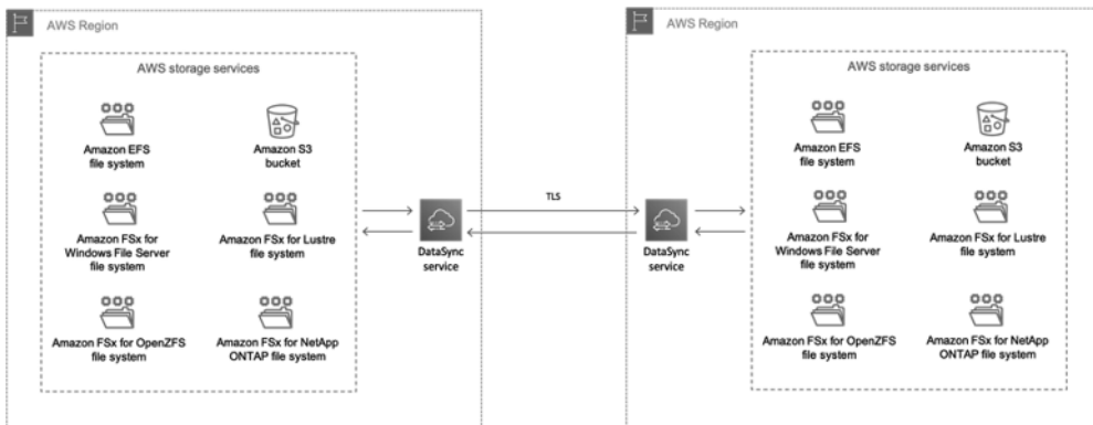
FIGURE 1.28 Transferring data between AWS storage services
