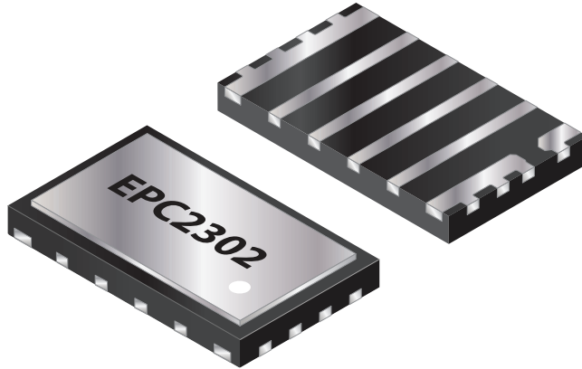
Figure 1.23 A finished packaged device in a PQFN format with exposed back surface for efficient heat extraction. This device measures approximately 5 mm × 3 mm. Source: With permission of EPC.
