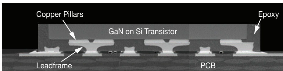
Figure 1.22 A GaN-on-Si transistor mounted inside an epoxy PQFN package. Source: With permission of EPC.
