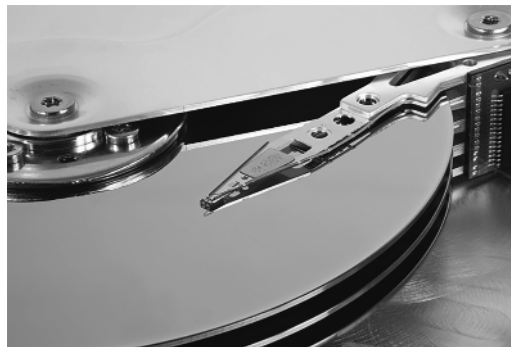
FIGURE 1.20 Inside a hard drive
