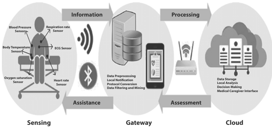
Figure 1.6 Generic architecture of IoT-based remote monitoring system.
