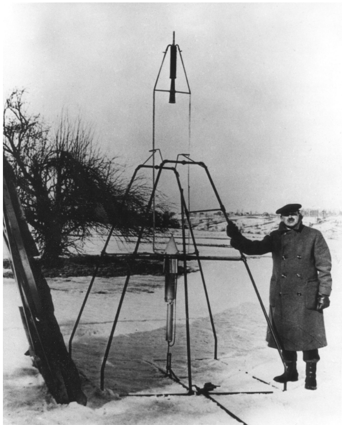
Figure 1.7 Robert Goddard's 1928 liquid-propellant rocket. Goddard is holding the trapezoidal launch frame of the rocket. (Source: NASA / Public domain.)
