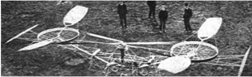
Figure 1.3 Paul Cornu's rotorcraft that made the first free-flight of a heavier-than-air rotorcraft. (Source: PD-USGov .)
