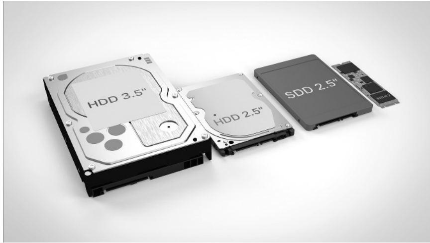
FIGURE 1.9 Four storage devices: a 3.5-inch HDD, a 2.5-inch HDD, a 2.5-inch SSD, and an M.2 SSD
