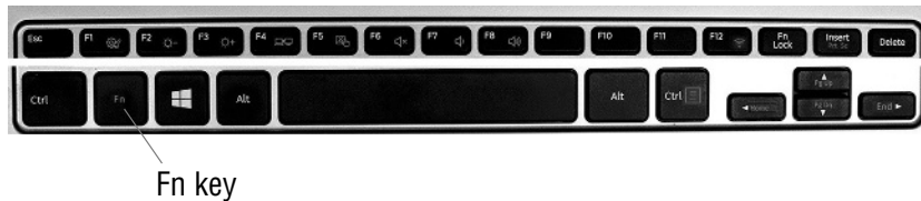
FIGURE 1.5 The top and bottom rows of a typical Windows laptop keyboard. Use the Fn key to activate the special laptop keys
