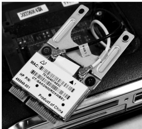
FIGURE 1.10 A wireless network card using the mini-PCIe interface
