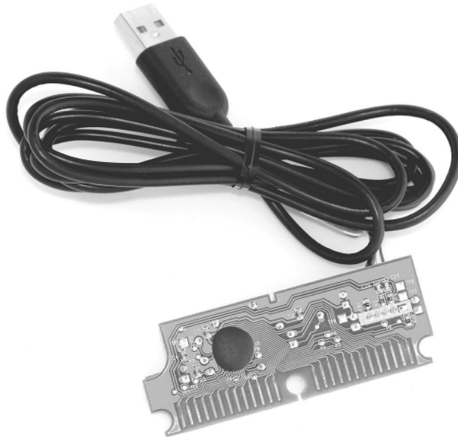
FIGURE 1-4: The insides of a keyboard, ready to be hacked.
