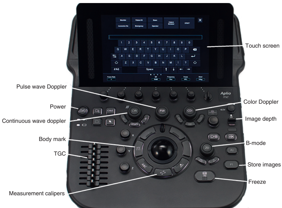
FIGURE 1.9 Knobology of ultrasound machine.
