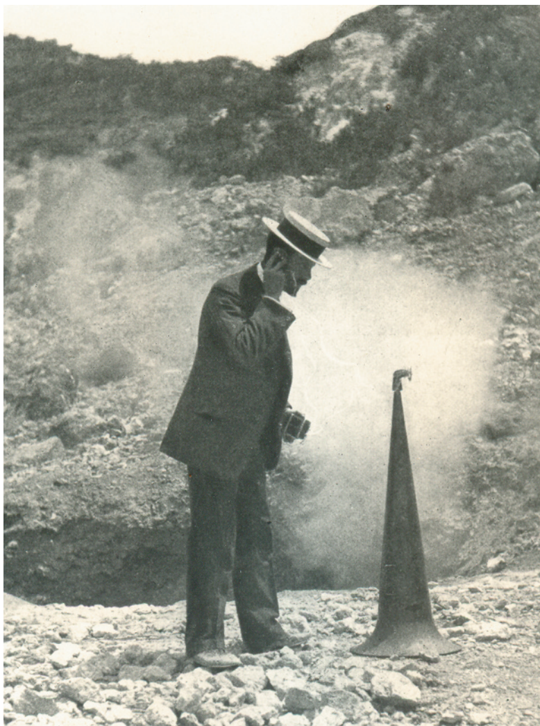
Fig. 1.24 F. A. Perret with an improvised “seismometer,” listening to subterranean noises at the Campi Flegrei, Italy. Photo from the US Library of Congress.
