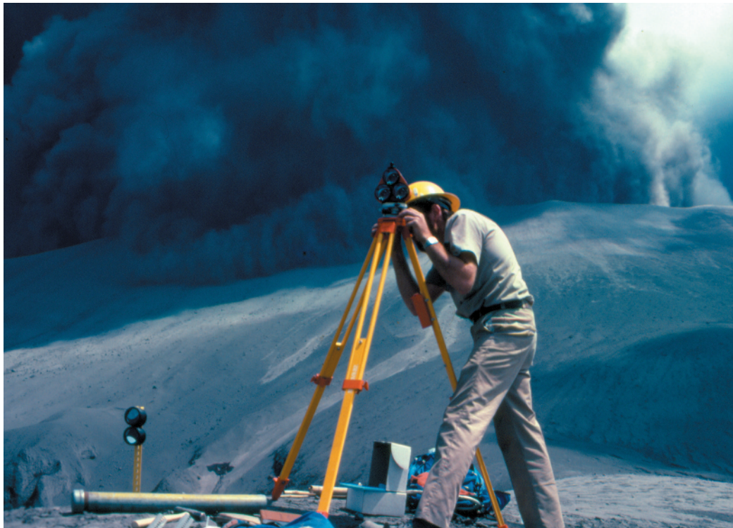
Fig. 1.8 EDM reflector at Pasir Bentang station below the erupting crater of Galunggung, August 1982. A small pyroclastic flow is beginning to cascade down the crater wall, and the thin deposits left by similar small Haws are seen behind the reflector tripod. Note the permanent reflector mounted on stake to left. Photo by Dedy Mulyadi.
