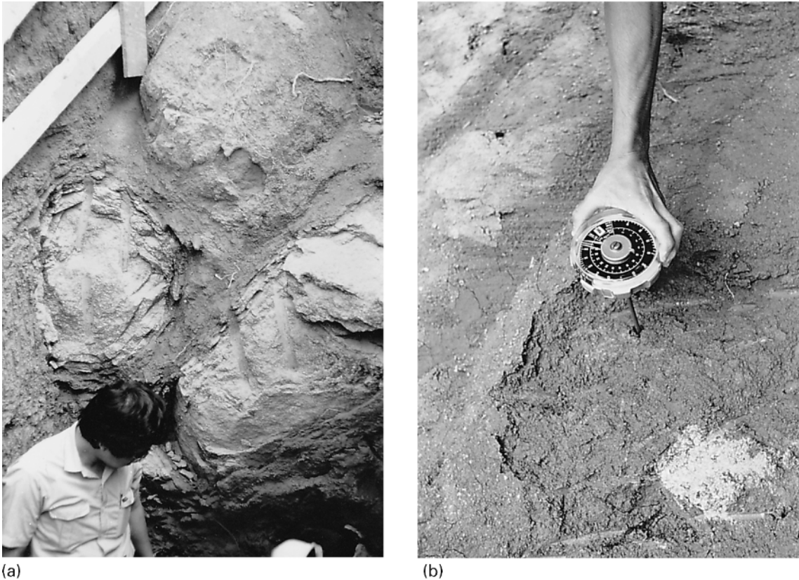
Fig. 1.12 (a) Granodiorite corestones showing exfoliated 'onion-skin' morphology in a tropical weathering zone of saprolite. (b) The hand-inserted shear vane is measuring the strength of a saprolite that was once solid granite—testament to the reality of rapid tropical chemical weathering. (Images from Tai Po, Hong Kong, courtesy of Steve Hencher.)
