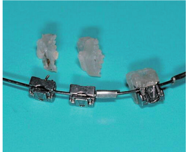
Fig. 1.12 Early Damon3 brackets. The mechanical linkage between the resin and metal components was subsequently strengthened to prevent this separation.
