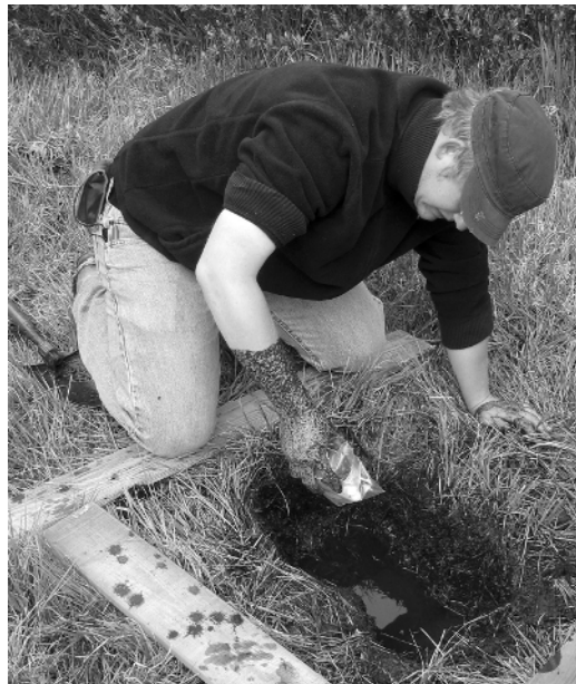
Figure 1-20. S. DeGraaf prepares to place a soil-temperature logger into a water-filled hole ~½m deep in a subalpine bog at ~3200m elevation, Colorado, United States. Study site is part of a long-term climate investigation. Photo by J.S. Aber.
