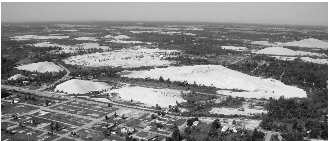
Figure 1-15. Huge chat piles are a legacy of lead-and-zinc mining at Picher, Oklahoma. Considered among the most seriously degraded sites in the United States, the landscape is essentially destroyed; toxic pollution of ground and surface water extends many kilometers downstream with severe impacts on human health and wetland habitats. View toward the southwest; blimp airphoto by J.S. Aber and S.W. Aber.
