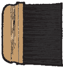
Fig. 1.81 Drag brush or brush grainer
