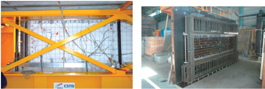
Figure 1.11. Shear wall specimen SHW3 (left figure) and shear wall reinforcement (right figure)
