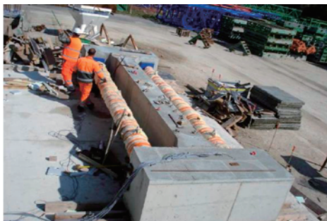
Figure 1.5. RG8 block with restrained shrinkage (I-shaped beam and steel struts)
