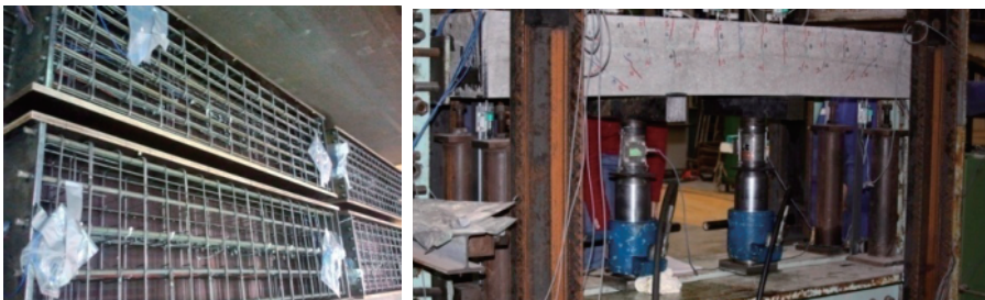
Figure 1.6. RL1- 1/3 scale beam under reinforcement
