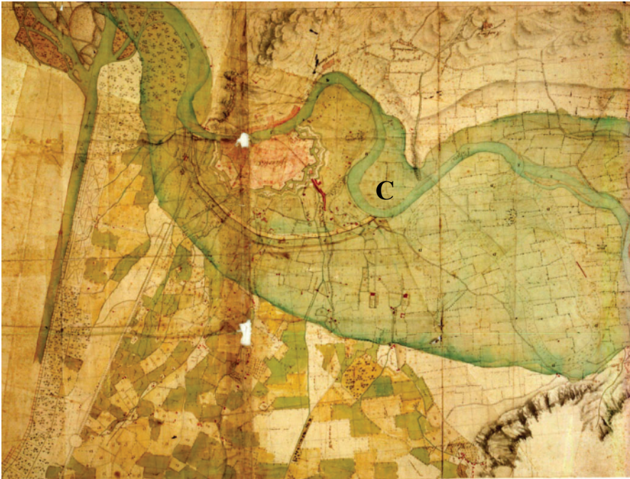
Figure 1.5. The Isère and the Drac in Grenoble in 1741. The Isère meanders and flows to the west (left); the Drac converges with the Isère downstream from the city (the Drac is dammed, but forms an alluvial fan in the northwest). The green area represents the spread of the flood on December 21, 1740; the outlet channel project bypassing Grenoble is represented (source: © Departmental archives of Isère). For full color image see: www.iste.co.uk/bravard/sedimentary1.zip
