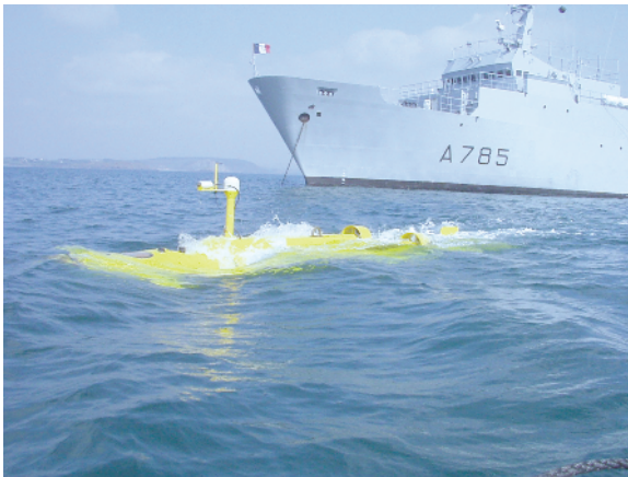
Figure 1.13. Redermor built by GESMA ( Groupe d'Etude Sous-Marine de l'Atlantique – Atlantic underwater research group ), on the water surface, still close to the boat it was launched from
