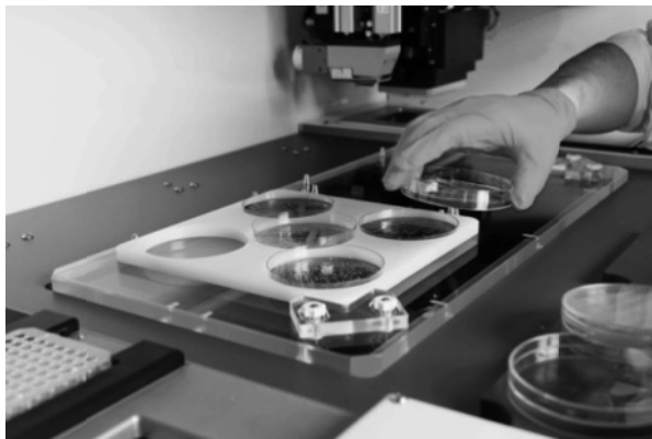
Figure 1.5. The colony picker is a piece of equipment that enables high-throughput screening of microbial strains possessing a particular property. It works by means of a camera that tracks colonies of microorganisms presenting a different phenotypic character (color, shape, pigment production, etc.)
