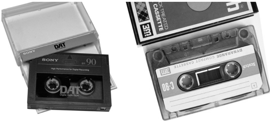
Figure 1.41. A DAT cassette (73 x 54 10.5 mm), on the left, compared to a mini-cassette (100 x 83 x 12 mm), on the right. For a color version of this figure, see www.iste.co.uk/reveillac/recording.zip
