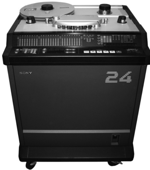
Figure 1.39. Sony PCM 3324 S digital multitrack (DASH 24 Tracks). For a color version of this figure, see www.iste.co.uk/reveillac/recording.zip
