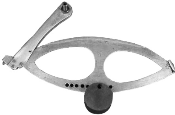
Figure 1.10. Pathé's "Poisson" Pantograph. At the left end is the engraving stylus and at the right end, the reproducing sapphire. At the bottom is the weight compensation and at the top, the rotation and holding axis
