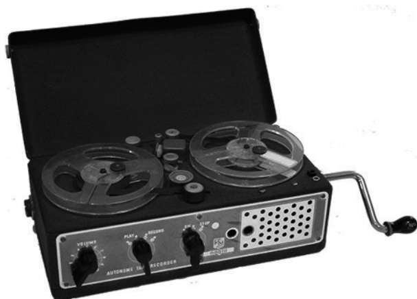
Figure 1.22. The Nagra I news reel-to-reel tape recorder with miniature lamps. For a color version of this figure, see www.iste.co.uk/reveillac/recording.zip
