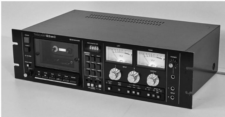
Figure 1.30. The Tascam 122 MKII professional cassette deck. For a color version of this figure, see www.iste.co.uk/reveillac/recording.zip
