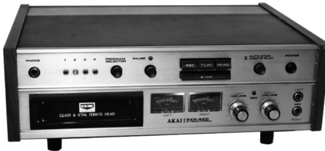
Figure 1.24. The Akai GXR-82D 8-track tape player/recorder
