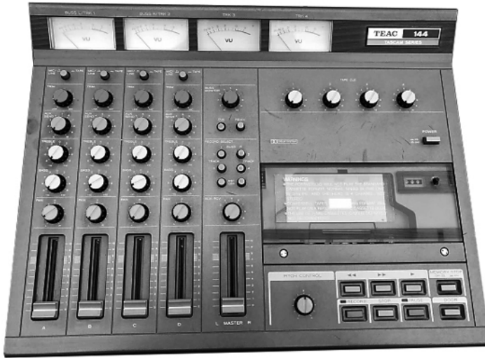
Figure 1.31. The Portastudio 144 stand-alone multitrack from Tascam (1979). For a color version of this figure, see www.iste.co.uk/reveillac/recording.zip
