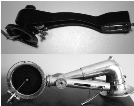
Figure 1.13. The electric pick-up (top) and the membrane read head (bottom)
