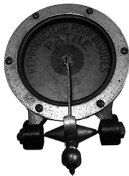
Figure 1.4. A Pathé sapphire pick-up for a vertically engraved disk. For a color version of this figure, see www.iste.co.uk/reveillac/recording.zip
