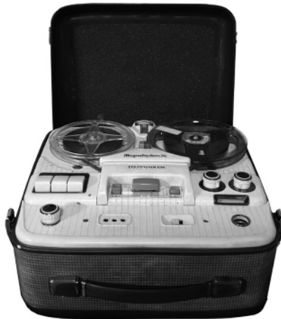
Figure 1.26. The Telefunken 76 (Tube) tape recorder, 4 tracks (stereo 2 X 2 tracks), speed: 4.75–9.5 cm/s, reel to 15 cm diameter, dating back to 1960. For a color version of this figure, see www.iste.co.uk/reveillac/recording.zip
