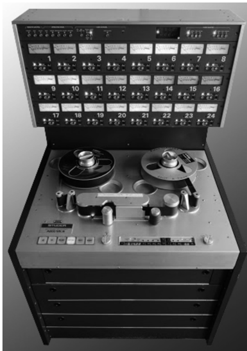
Figure 1.34. A 24-track 2-inch multitrack (Studer A800 – MKII), a standard of excellence in the studios of the 1970s and 1980s. For a color version of this figure, see www.iste.co.uk/reveillac/recording.zip
