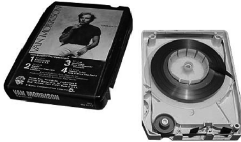
Figure 1.23. An 8-track tape and its internal structure. For a color version of this figure, see www.iste.co.uk/reveillac/recording.zip
