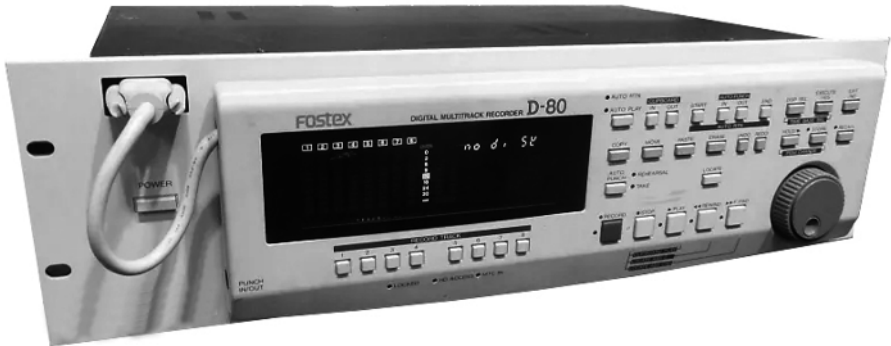
Figure 1.49. The Fostex D80 hard disk recorder – 8 tracks (1996). For a color version of this figure, see www.iste.co.uk/reveillac/recording.zip
