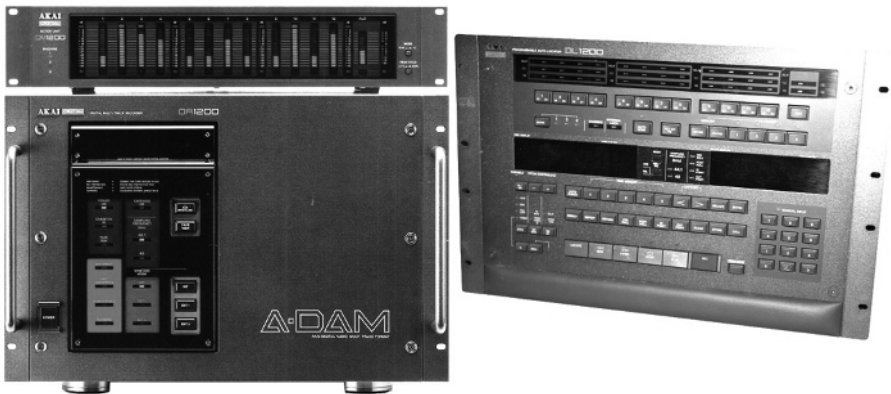
Figure 1.48. The imposing Akai DR1200 reader-recorder with its bank of vu-meters (DM 1200) and its locator (DL 1200). For a color version of this figure, see www.iste.co.uk/reveillac/recording.zip
