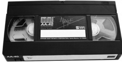
Figure 1.45. An S-VHS tape for use with an ADAT recorder. For a color version of this figure, see www.iste.co.uk/reveillac/recording.zip
