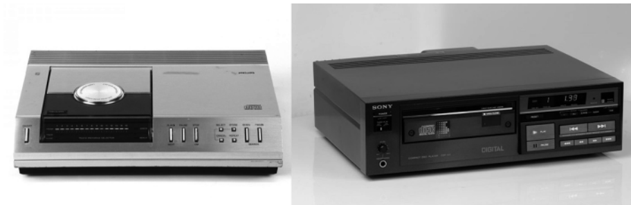
Figure 1.36. The first two commercial CD players, the Philips CD100 (left) and the Sony CDP-101 (right)
