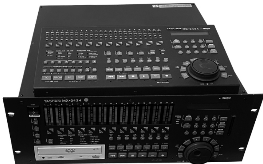
Figure 1.50. Tascam MX-2424 – 24-bit, 96 kHz, 24-track hard disk recorder (2004) with its RC2424 remote control. For a color version of this figure, see www.iste.co.uk/reveillac/recording.zip
