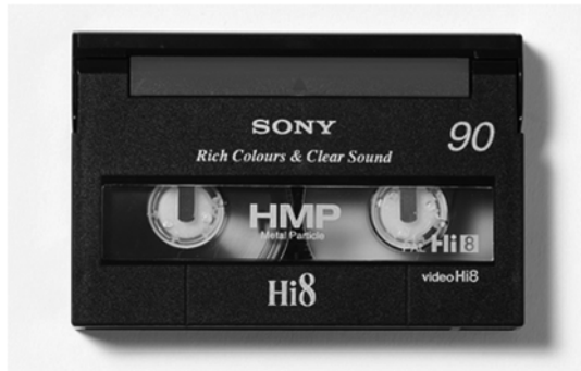
Figure 1.47. A 90 minute Hi-8 cassette (95 x 62 x 15 mm). For a color version of this figure, see www.iste.co.uk/reveillac/recording.zip
