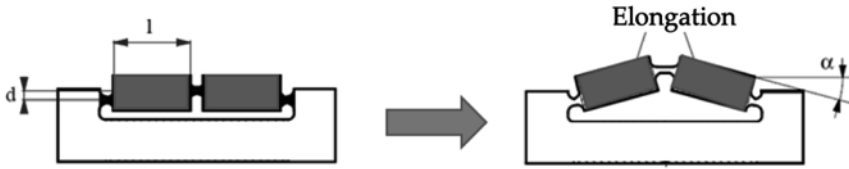
Figure 1.5. Displacement amplification under stress
