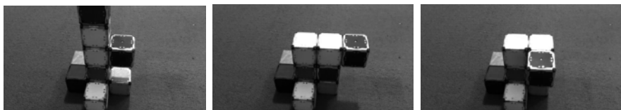
Figure 1.46. Example of 4D printing using cubes (according to Sussan (2014))
