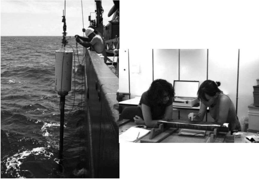
Figure 1.28. Sampling and exploitation of deep-sea sediment cores on board an oceanographic vessel
