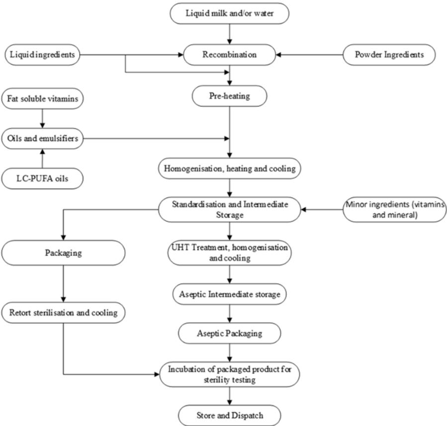
Figure 1.2. Schematic representation of the manufacture of liquid infant formulae (Montagne et al. 2009)
