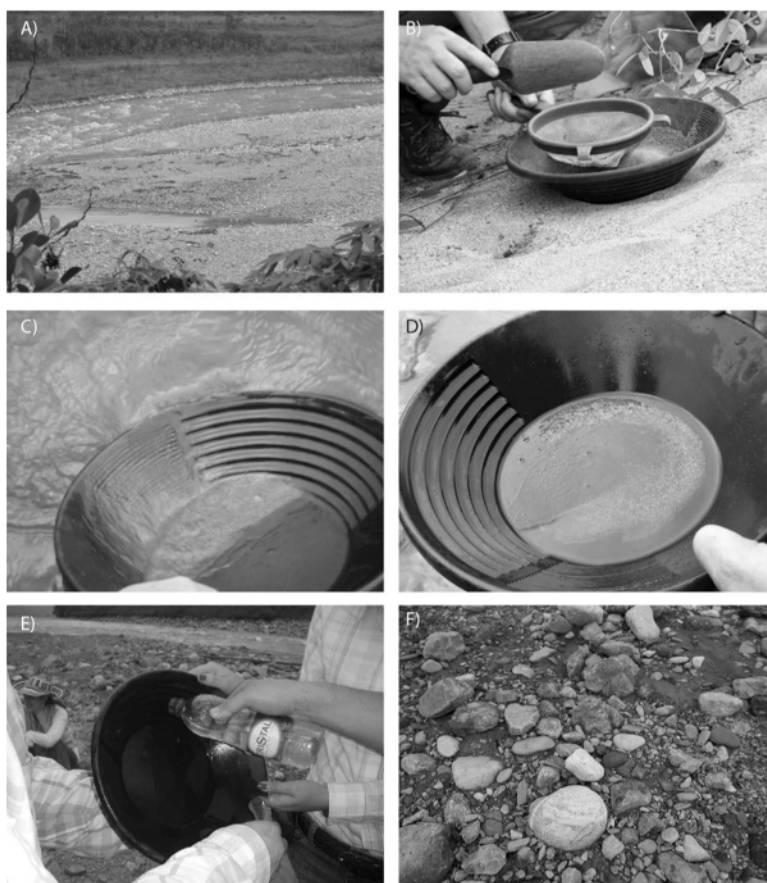
Figure 1.6. Sampling of modern river sediments for detrital fission-track studies. (A) Selection of sampling site will in many cases depend on access. Gravel and/or sand bars along the river bank are preferable. If possible, heavy mineral placer deposits can be used. (B) Sieve sediment to eliminate very coarse sand and gravel. (C and D) Wash out all mud and reduce the light mineral fraction to concentrate heavy minerals, which is in many locations black (magnetite) and/or red (garnet). Apatites and zircons will be in this fraction. (E) Transfer sample material into bag and repeat the whole procedure 8–10 times to collect about 200 g of sample material. (F) Take note of all the lithologies in the drainage basin represented in the river gravels and boulders. Also record the sampling location with GPS coordinates and/or on a map. For a color version of this figure, see www.iste.co.uk/jolivet/fission.zip
