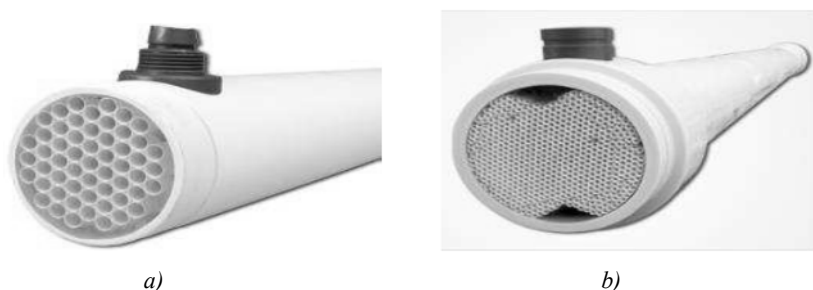
Figure 1.15. Examples of membrane modules operating: a) in cross flow; b) helped by an airlift
