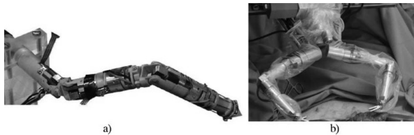
Figure 1.5. Architectures with rigid links and discrete joints: a) DRIMIS (ISIR) [SAL 04]; b) SPRINT (Araknes project) [PIC 10, SAN 11]
