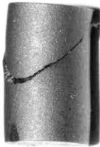
Figure 1.9. Specimen made of VT20 titanium alloy fractures in compression testing
