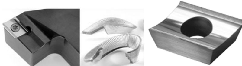
Figure 1.14. Shear Geometry® cutting tool, formed chip and high-rake insert (Robertson Precision, Inc (Redwood City, CA))
