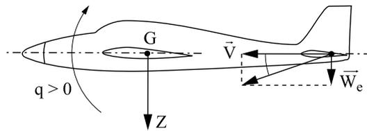
**Figure 1.17.** Modification of the elevator attack angle due to angular pitch velocity
