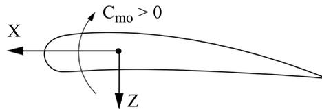
**Figure 1.24.** *For a "normal" profile section, the static momentum is positive*
