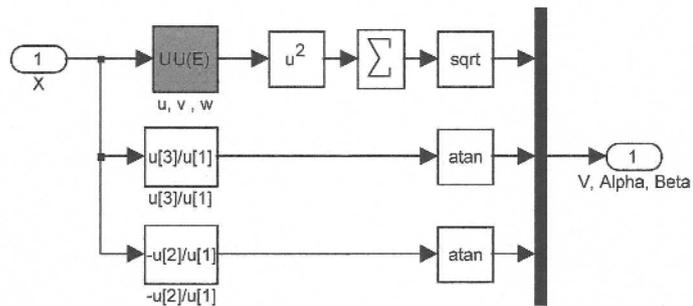
Figure 1.10. SIMULINK scheme to compute  $V$ ,  $\alpha$  and  $\beta$
