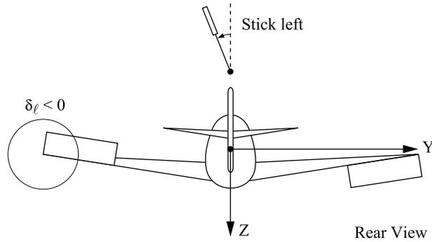
**Figure 1.19.** The control stick moves to the left, the left aileron goes up and the right aileron goes down, the plane to make a left roll
