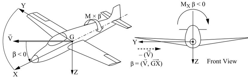
Figure 1.18. Roll torque  $M_x$  due to side slip angle  $\beta$
