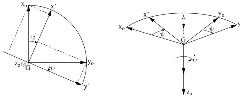
**Figure 1.2.** First Euler rotation  $\psi$  around the  $Gz_0$  axis
