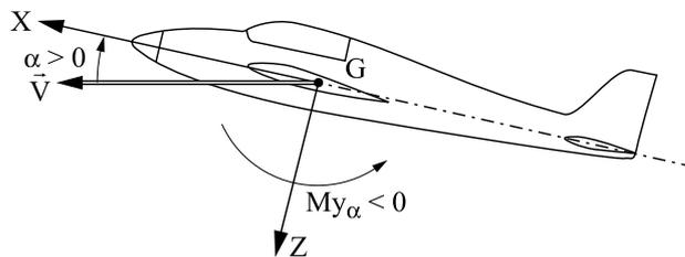
**Figure 1.21.** The horizontal fin creates a torque on the opposite side of  $\alpha$
