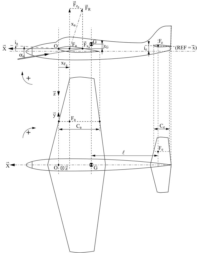
Figure 1.45. Geometrics of the wing and the horizontal stabilizer
