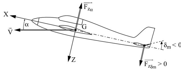
**Figure 1.16.** *Vertical lift due to elevator control surface angular displacement*
