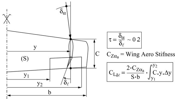
Figure 1.52. The figure above shows the half-wing planform
