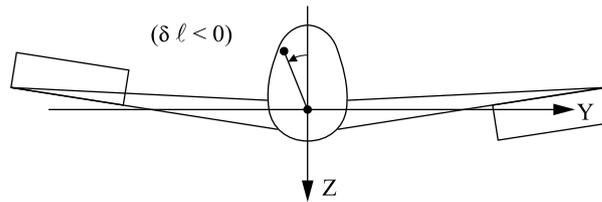
**Figure 1.11.** Aileron stick displacement to the left side, where the left aileron goes up and the right aileron goes down. (Rear view)
