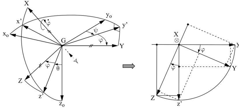
Figure 1.4. Third Euler rotation  $\phi$  around the GX axis
