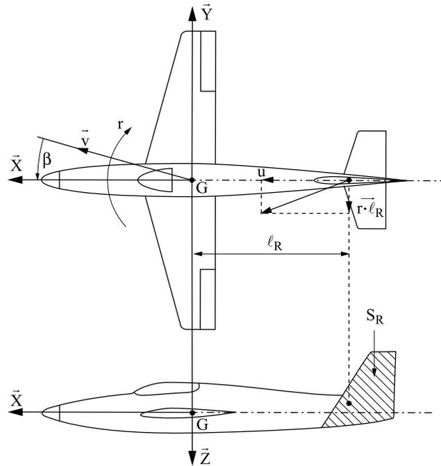
Figure 1.59. Parameters of yaw stiffness and yaw damping
