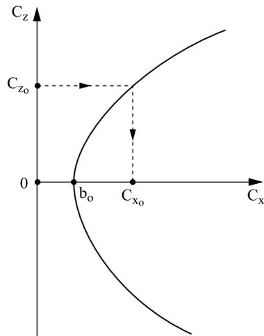
**Figure 1.50.** The Lilienthal polar plot  $CZ$  as a function of  $CX$  by the body reference
