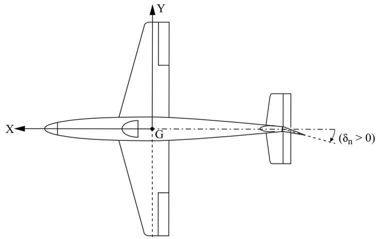
**Figure 1.13.** *Left displacement of the yaw control surface*
