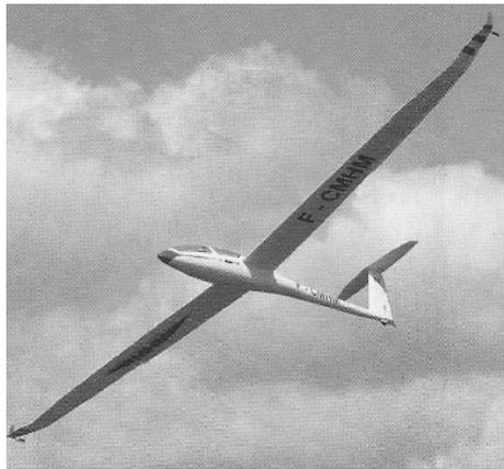
**Figure 1.54.** A glider with high-aspect ratio wings
