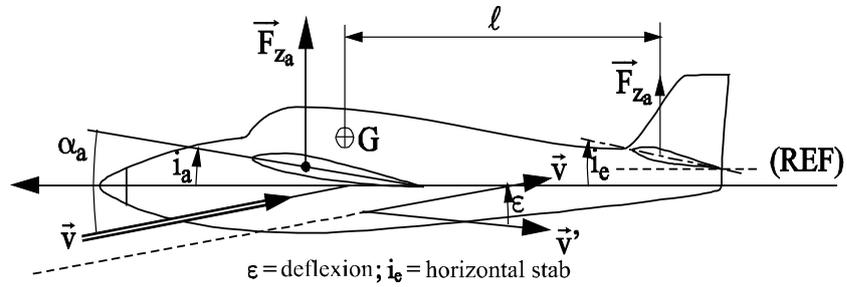
Figure 1.46. Figure showing angular deviations of wing and stabilizer
