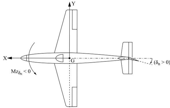
**Figure 1.26.** Rudder control surface motion creates yaw torque
