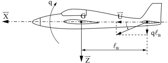
**Figure 1.56.** Change of attack angle at the stabilizer due to  $\vec{V}$  and  $q$
