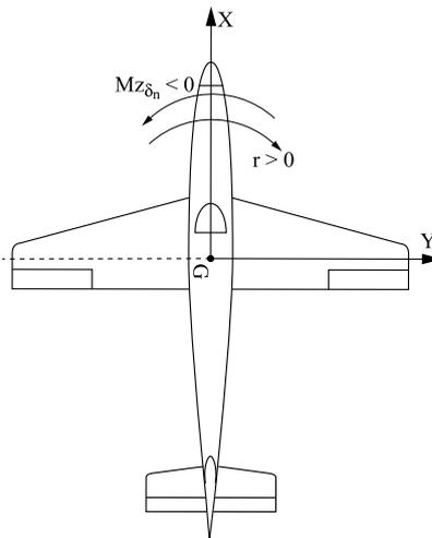
**Figure 1.27.** Yaw angular velocity creates an opposite damping torque
