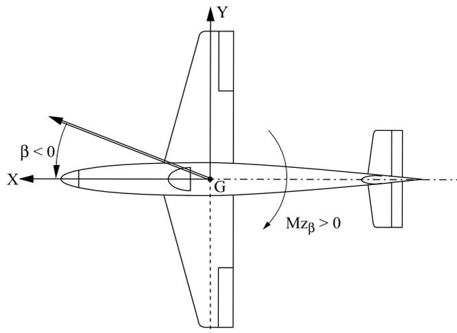
**Figure 1.25.** The directional stability aligns GX with the velocity vector
