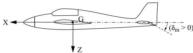
**Figure 1.12.** Elevator stick displacement to the front, where the elevator control surface goes down
