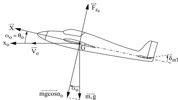
**Figure 1.47.** An elevation time  $\delta_{mT}$  is necessary to maintain an attack angle  $\alpha_0$
