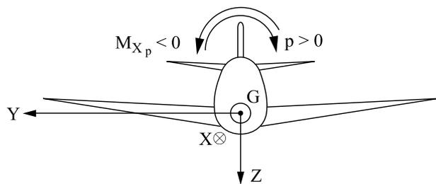
**Figure 1.20.** The damping torque  $M_{Xp}$  is on the opposite side of  $p$
