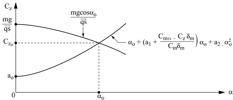
Figure 1.48. Graphical solution to obtain  $\alpha_0$
