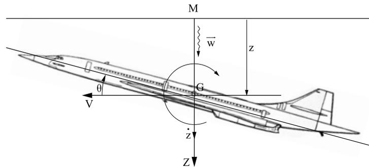
**Figure 1.40.** Lateral figure of Concorde, showing altitude  $z$  and Pitch angle  $\theta$
