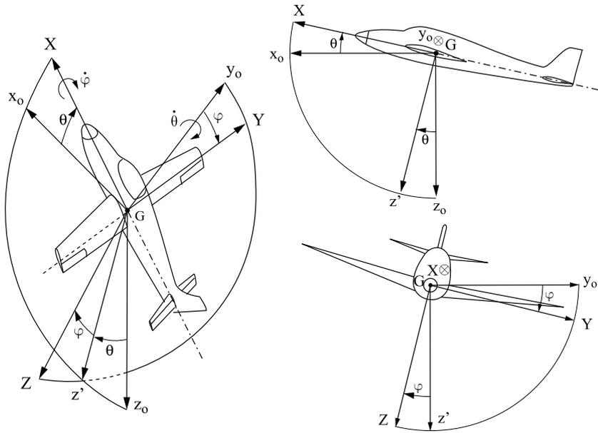
Figure 1.32. Angular positioning by the horizontal plane  $Gx_0y_0$
