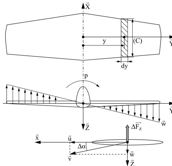
**Figure 1.53.** The change of attack angle along the side of the wingspan due to roll angular velocity
