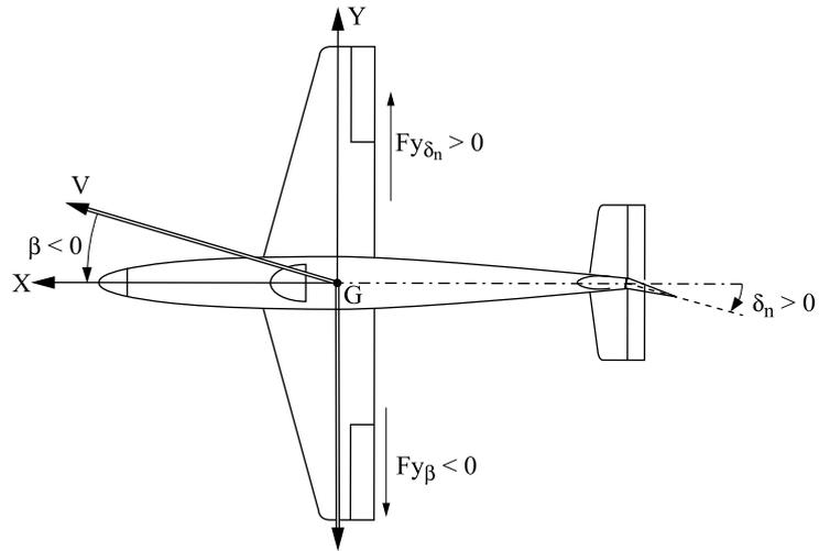
**Figure 1.15.** Dependence of Side Lift on  $\beta$  and  $\delta_n$
