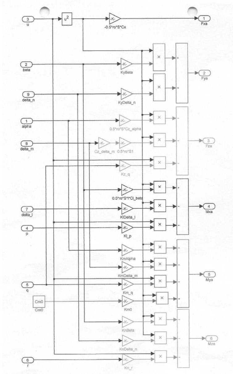
**Figure 1.29.** SIMULINK diagram. All the necessary inputs are displayed on the left side, and the six outputs are displayed on the right side
