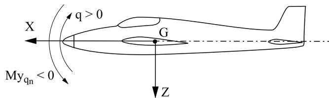
**Figure 1.23.** *Pitch torque and angular velocity are opposite*
