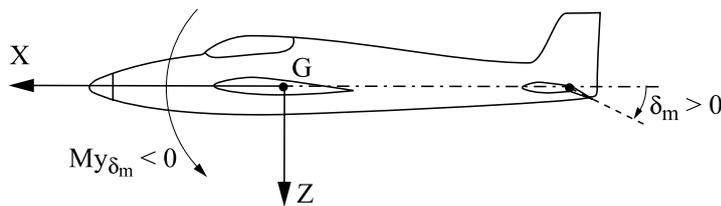
**Figure 1.22.** For an elevator control surface motion going down, the pitch torque is negative
