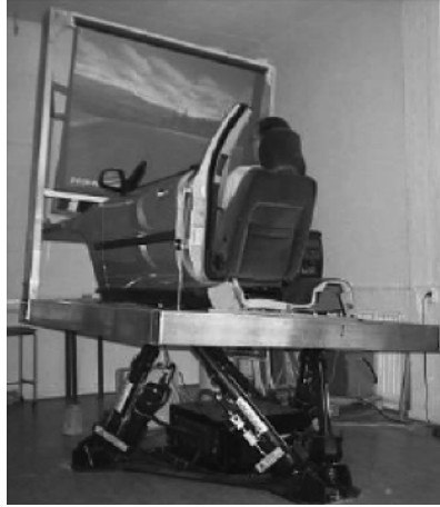
Figure 1.4. Parallel platform simulator at the Chalmers University – Sweden
