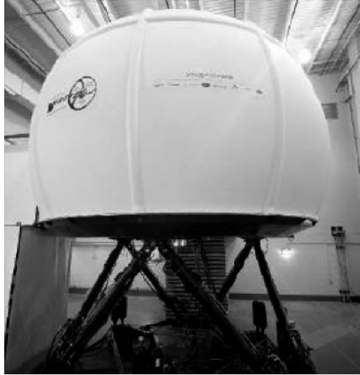
Figure 1.6. Gough–Stewart platform simulator of the VIRTTEX – USA
