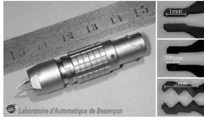
**Figure 1.5.** Example of *Microprehensile Microrobot On Chip (MMOC)* and its *Nickel effector parts [AGN 05]*
