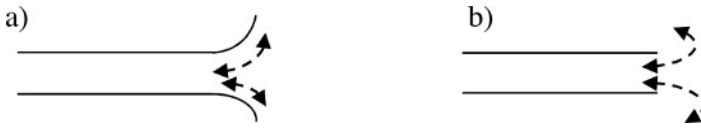
Figure 1.5. a) The radius of curvature of an open end of a guide is larger than acoustic displacement (dashed arrow). b) The radius of curvature of an open end of a guide is smaller (sharp end) than the acoustic displacement. The fluid displacement (dashed arrow) does not follow the wall and vortex shedding occurs
