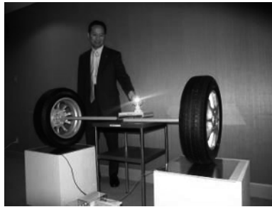
Figure 1.13. a) Diagram of the power transfer system proposed by Toyohashi University of Technology, Japan [HAN 11]; b) experimental setup
