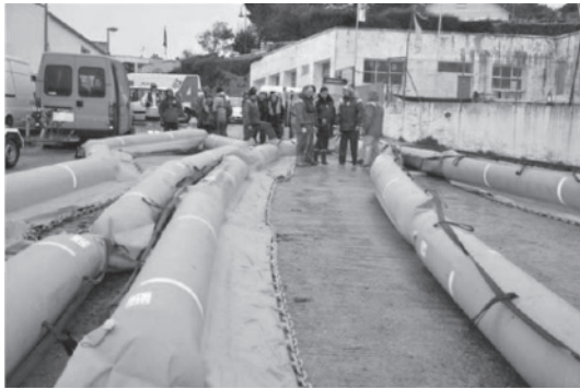
Figure 1.6. Inflated floating part and undersea skirt part of a boom
