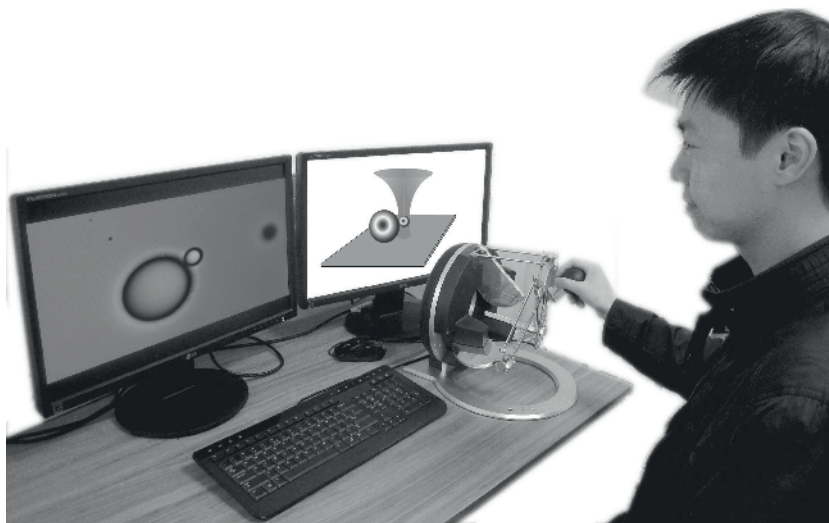
Figure 1.1. Dextrous use of a micromanipulation platform. An optical trap is teleoperated with an interface that allows force measurement feedback to be haptically experienced. A 3D reconstruction of the scene can also increase user immersion. The haptic interface presented is the Omega TM from Force Dimension. For a color version of this figure, see www.iste.co.uk/ni/tweezers.zip
