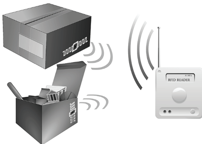
Figure 1.1. Operation schema of an RFID system. The reader, most often linked to a database, questions the tag, located here on a packing box. In this way, the reader can recover the tag's ID, contained in the RFID chip located in the center of the tag
