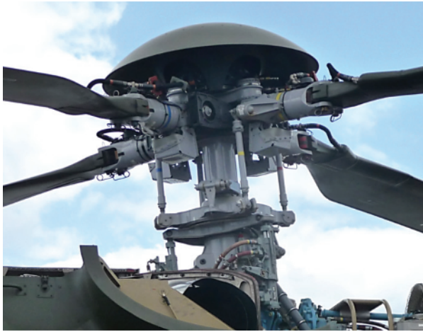
Figure 1.3. Swashplate actuation on an AS332 helicopter
