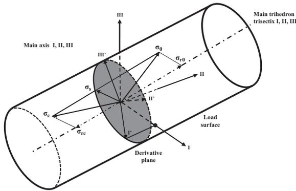
**Figure 1.2.** Space of the principal stresses in the Von Mises cylinder with the state decomposition of depressive ( $\sigma_D$ ) and compressive stress ( $\sigma_C$ ) accompanied by its deviatoric ( $\sigma_S$ ) and spherical components ( $\sigma_{TD}$  and  $\sigma_{TC}$ )
