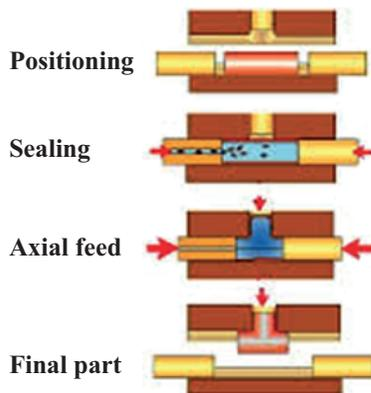
**Figure 1.3.** *Hydroforming principle*
