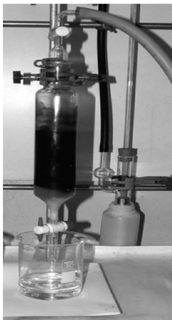
Figure 1.18 Experimental apparatus for decolorizing ionic liquids [71].
