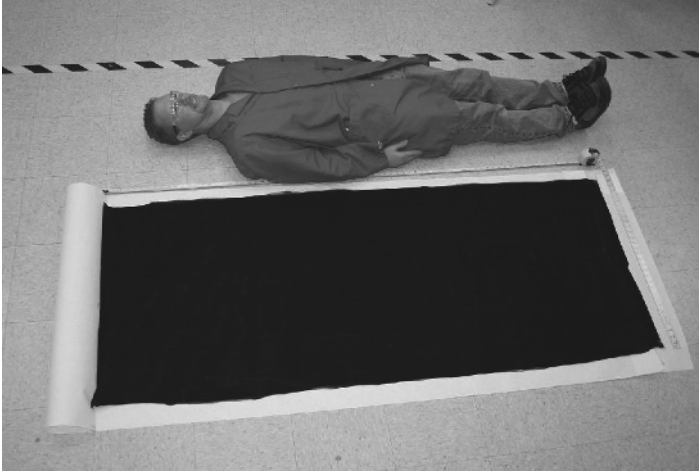
Figure 1.2 Nanocomp’s 3’ × 6’ sheet made from carbon nanotubes set a world size record. The company is refining processes to manufacture these sheets, which can be up to 100 times stronger than steel, in commercial
