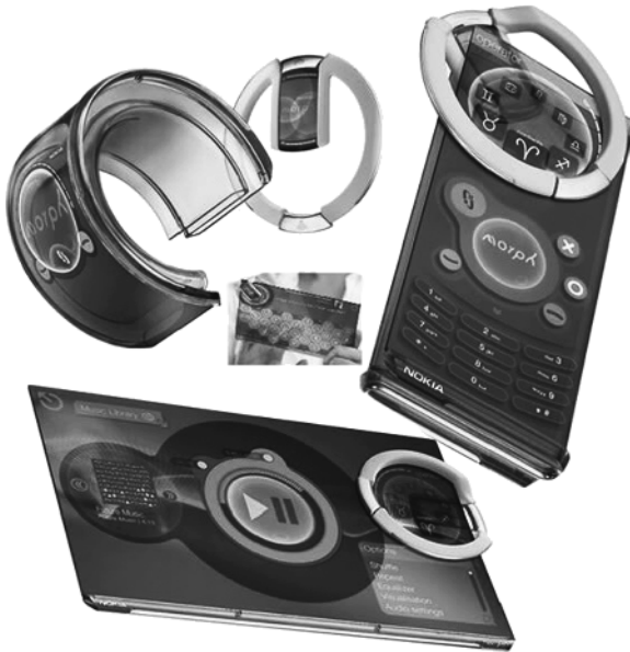
Figure 1.4 Nokia's Morph concept phone uses nanotechnology to give the cell phone a new form factor that includes “shape shifting” (image courtesy of Nokia).
