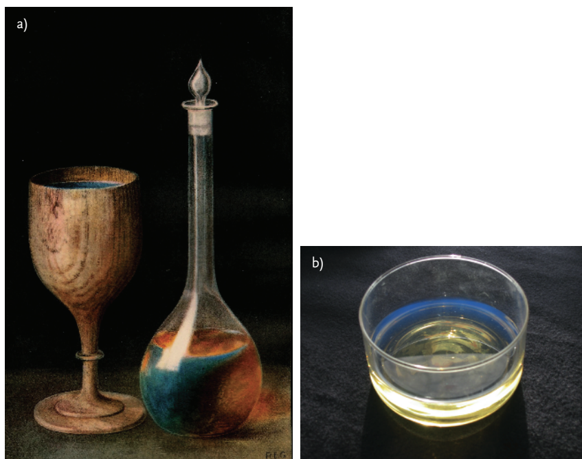
Figure 1.2 Absorption and fluorescence colors of an infusion of Lignum nephriticum under day light. (a) taken from Safford, W.E. (1915) Ann. Rep. Smithsonian Inst. , 1915,
