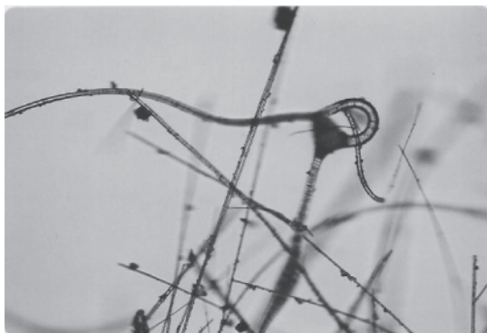
Figure 1.8 An example of an indoor aerosol of solid particles (dust aerosol). The whorl on the fibre in the foreground (upper right) is about 25\ \mu\text{m} in diameter. Photomicrograph by the author.
