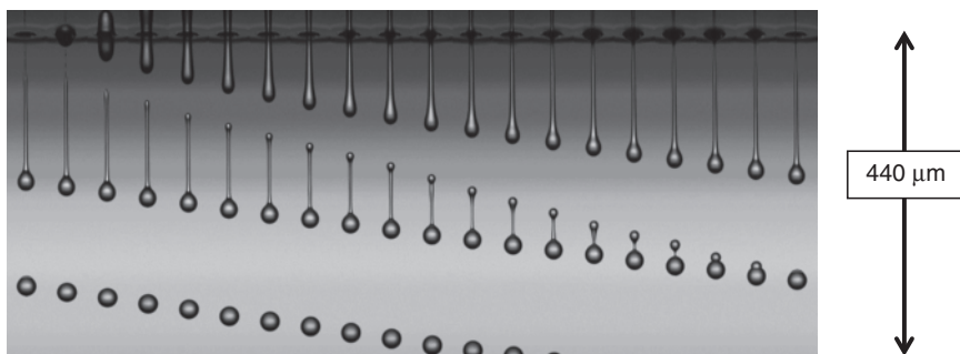
Figure 1.3 Jetting of a high viscosity ink from a prototype print head (Océ Technologies, Venlo, the Netherlands) with a nozzle of 27\text{ }\mu\text{m} diameter and driven at 20\text{ kHz} with a positive pulse [5]. The ink is silicon oil with viscosity of 9.3\text{ mPa s} , density 930\text{ kg m}^{-3} and surface tension 20.2\text{ mN m}^{-1} . The images were obtained by using a dual-cavity Nd:Yag laser (wave length 532\text{ nm} ) and fluorescent diffusor to remove any coherence in order to end up with images free of any speckle and interference fringes [6]. The pulse time of the flash has a duration of 8\text{ ns} . The picture is a concatenation of images taken with increasing delay from the leading edge of the pulse with steps of 2.5\text{ }\mu\text{s} . The droplet speed after the tail has merged with the main droplet is 3\text{ m s}^{-1} . The droplet size measures 9.3\text{ pl} . Source: With permission from van der Meulen 2015 [5].
