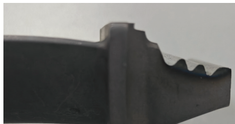
Figure 1.9 Typical grinding burn on fir-tree turbine blade root surface.
