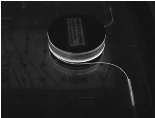
Figure 1.13 Erbium doped fiber glowing in the dark, upon excitation by the pump radiation at 980 nm. Please find a color version of this figure on the color plates.
