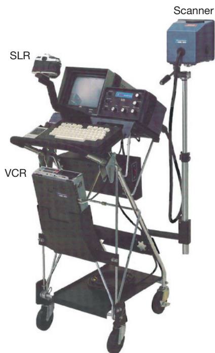
Figure 1.81 Liquid-nitrogen-cooled Inframetrics 535 IR camera from 1980s producing images of 130 \times 200 pixels. The camera was cooled with liquid nitrogen (funnel on top). Hard copy recording was performed on 35 mm film (photo of computer screen) and half-inch VCR (VHS). The needed floor area of 17.5 \times 22.5 \text{ in}^2 was advertised as space saving (see Inframetrics PDF brochure from FLIR web site [209]).
