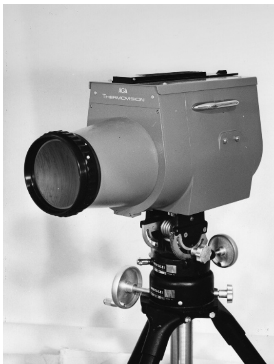
Figure 1.80 AGA Thermovision 665 camera This camera type was sold starting around 1965. Image courtesy FLIR systems, Inc. (2016).
